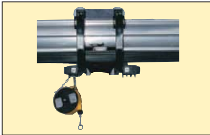
External crab (EC) for mechanical nozzle with vise grip, balancer and suspension belt.
